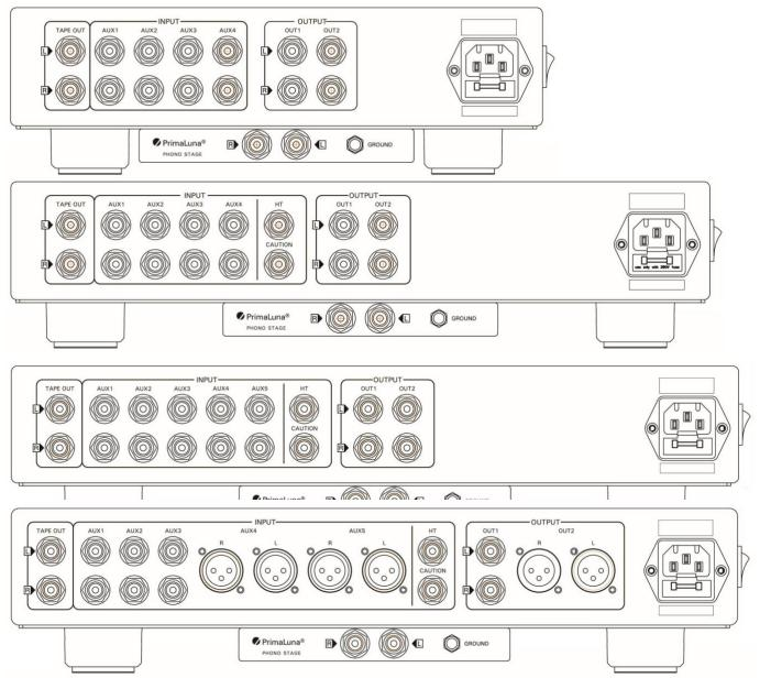
At the rear panel, you will find your inputs, eventually the HT Pass-Thru, Tape Out and preamp outputs.
