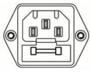
**Mains Fuse:** The mains fuse is located on the rear of the preamplifier, just below the power cord socket (see picture on the left). The fuse rating is 1 x Littelfuse 213 Series 1A Slow Blow 5 x 20mm fuse for 100-125VAC and Littelfuse 213 Series 0.5A Slow Blow 5 x 20mm fuse for 200-250VAC. Always replace with the same type and value fuse! The fuse holder can be opened using a small slotted flat blade screwdriver.
