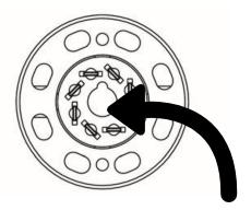
Some tubes and tube sockets have a "center key" which must line up! If you misalign them and use brute force, you will damage important and expensive parts of your amplifier!!
